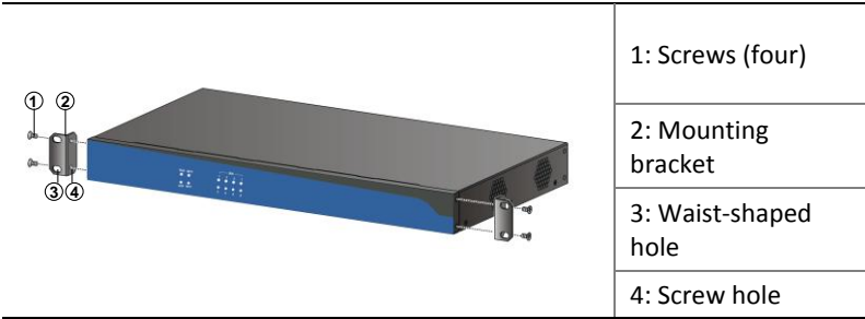
Figure 2-2 Installing the mounting brackets
